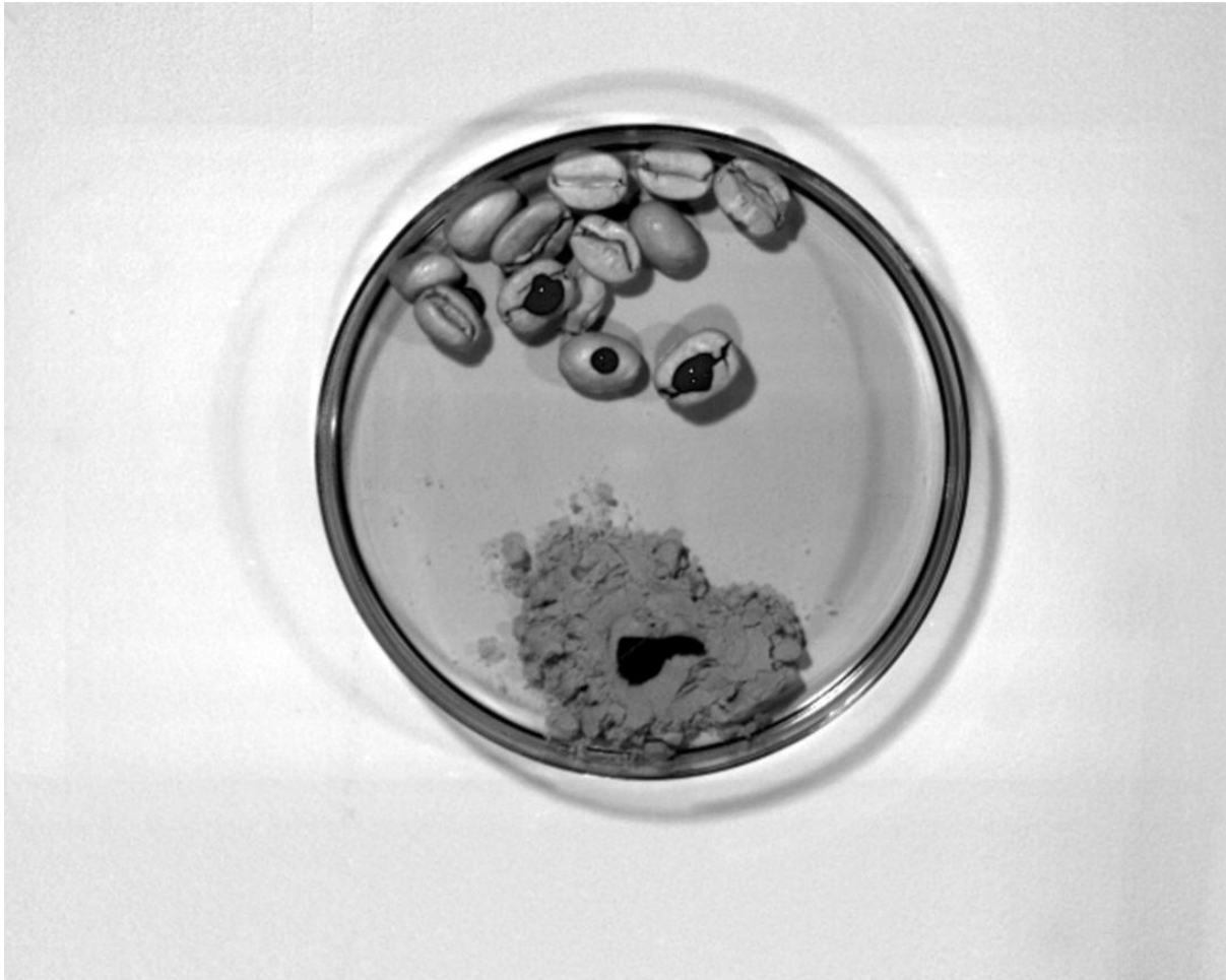
SWIR 1920 nm image shows water contrast on coffee beans. Image: Emberion
